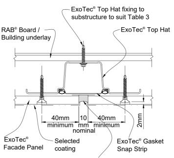
Joint sealant over bond breaker tape for 4.0 kPa wind pressures and above, refer to ExoTec® Facade Panel Technical specification for suitable flexible sealant.
